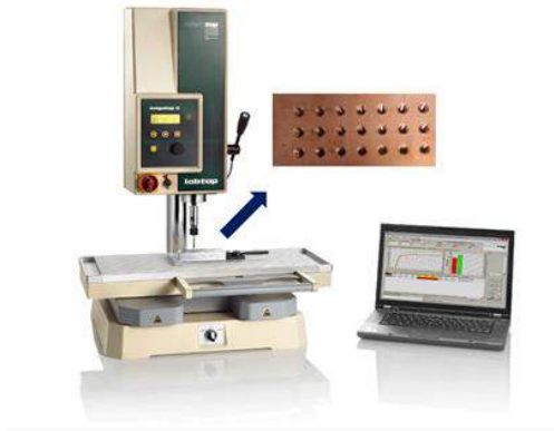
Figure 2. Tapping Torque Test System
