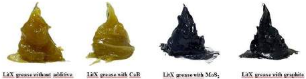
Fig. 5. Appearances of LitX grease and LitX greases formulated with different additives.
