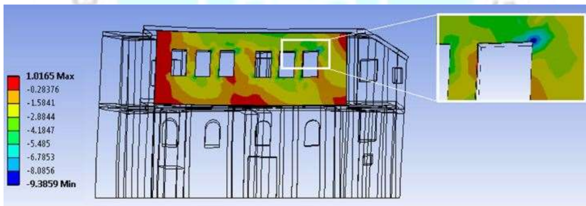
Fig. 18. Compression Stresses (MPa)
