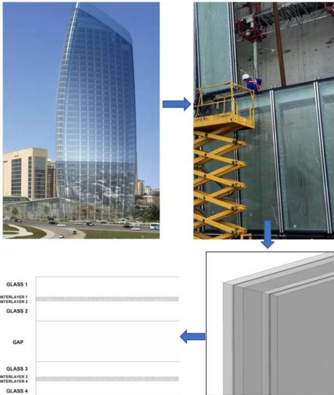
Figure 1. Components of the Glass Panel
